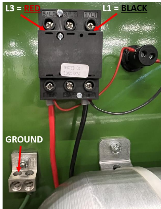
Internal switch wiring locations for power input
